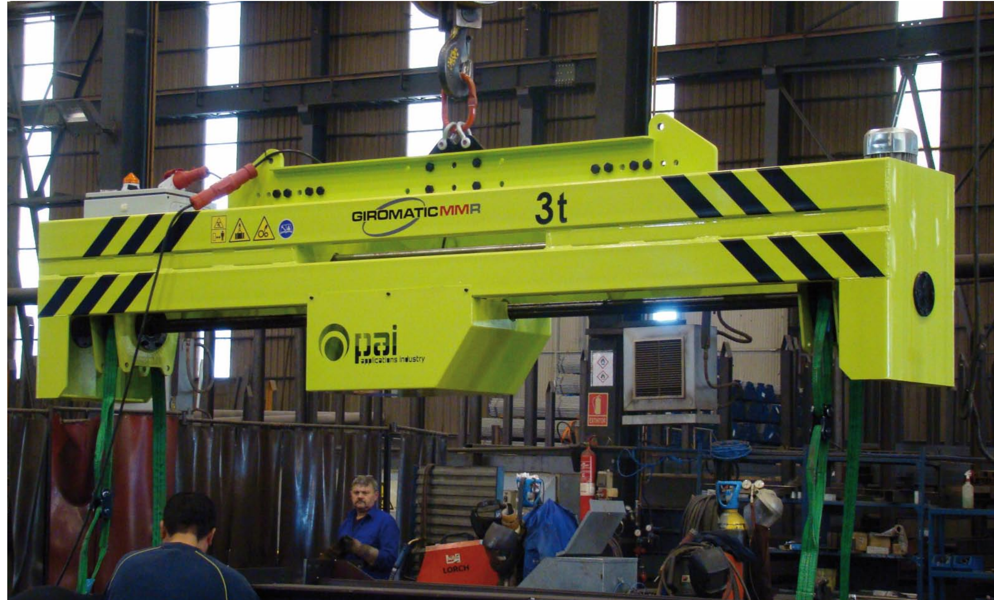
GIROMATIC MM-R, distance between pulleys with regulation GIROMATIC MM-R, distancia entre poleas regulable
