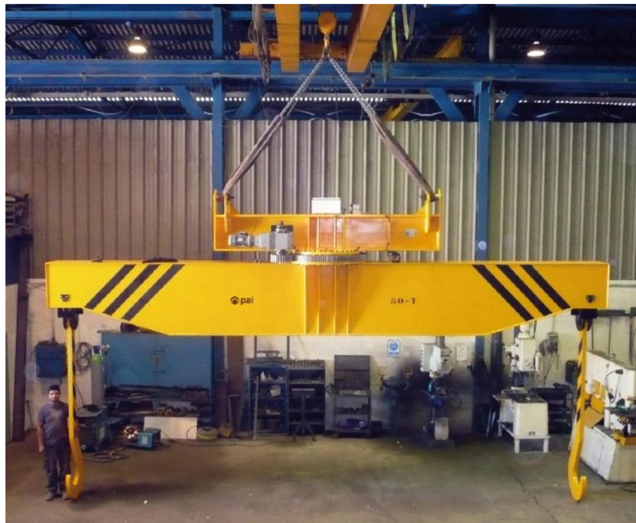
Spreader with rotator system integrated Balancín con sistema de giro
