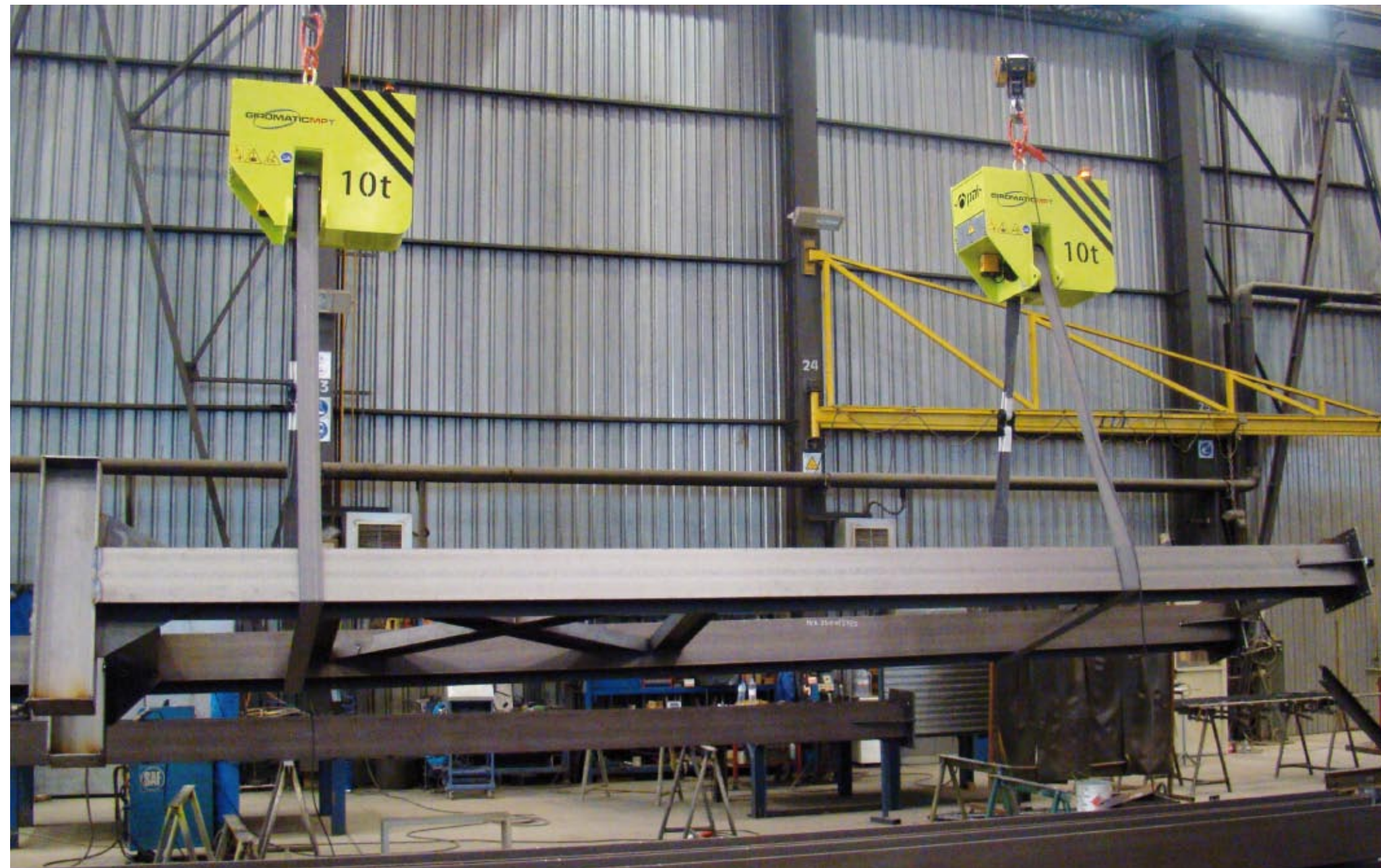
GIROMATIC MP C/T suspended from crane GIROMATIC MP C/T suspendido de una grúa
